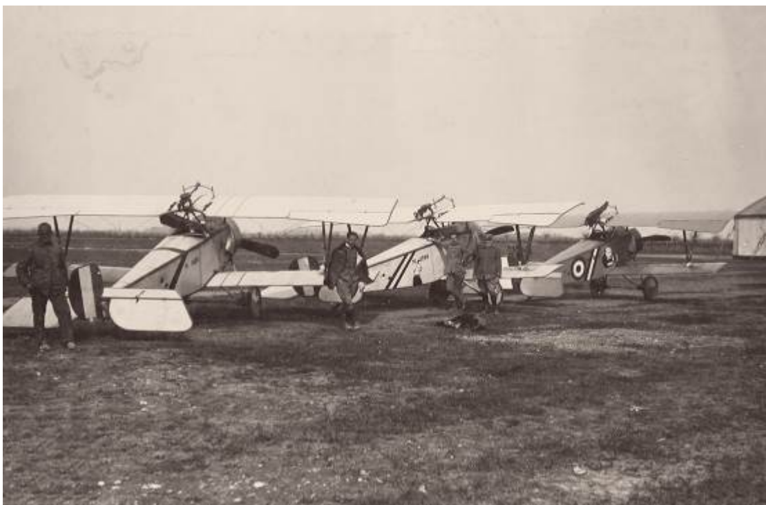
76 a Squadriglia Nieuport Ni.11s at Borgnano, Isonzo front, in early 1917. The aircraft are equipped with a Lewis machine-gun that is not synchronized.
