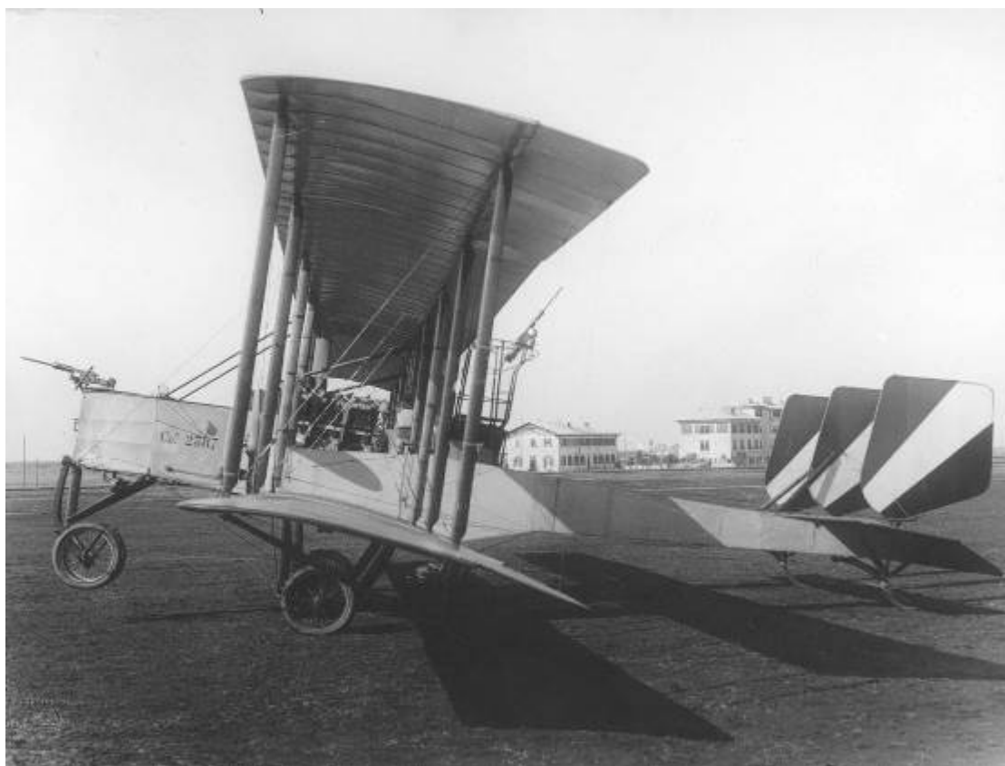
Spring 1917, a 450-hp Caproni Ca.3 bomber from the 9 a Squadriglia. The forward and rear machine-guns, both 6.5 mm FIAT-Revelli, are clearly visible.
