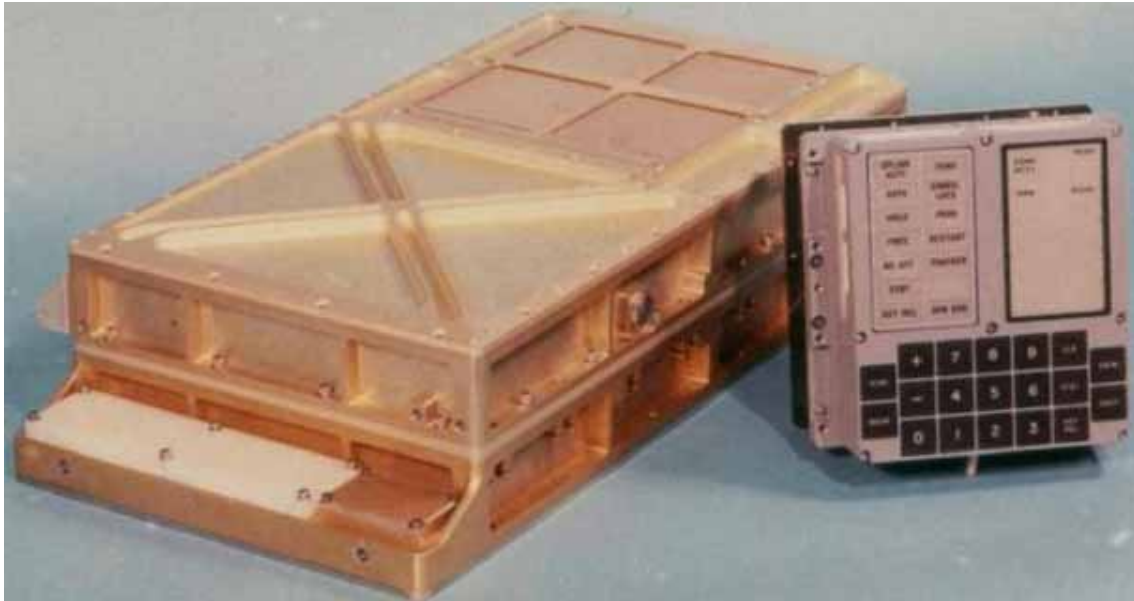
Figure 11 : Apollo Guidance Computer (AGC)
